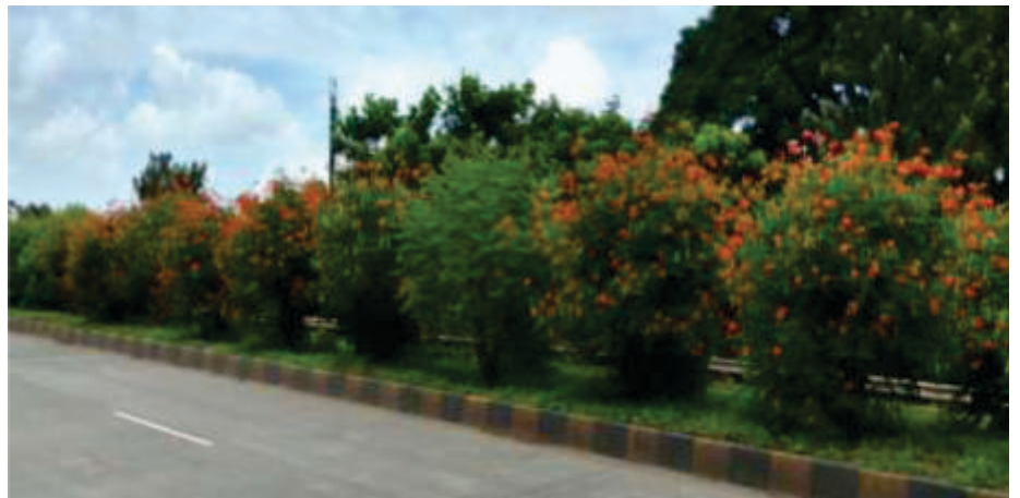
Figure 16: Caesalpinia planted along median acting as anti-glare screen; through proper pruning, can be maintained as effective anti-glare hedge
