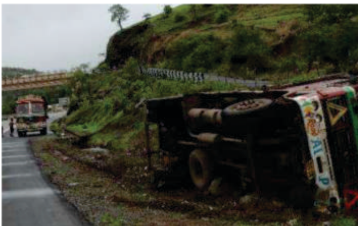
Figure 3: Truck driver wanting to park his truck on the shoulder did not notice the narrowing shoulder. Truck toppled over to the left
